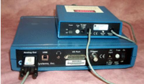
2. Plug the **BSLSTM Reference Output** connector into **CH 2** of the **MP3X** unit.
