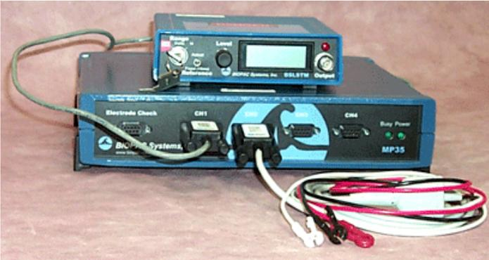
BSLSTMB Reference cable, SS2L lead and HSTM01 stimulating probe connections
